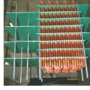
Water tank evaporator
